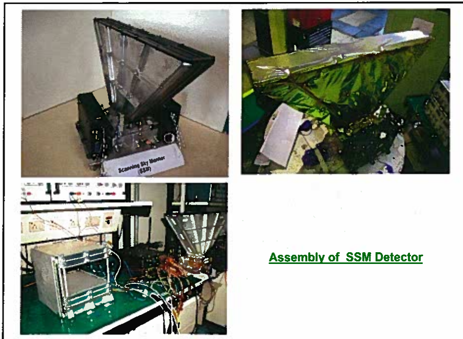
Fig 12 : Views of individual Position Sensitive Proportional Counters used in SSM at different stages of assembly (courtesy- SSM team).
