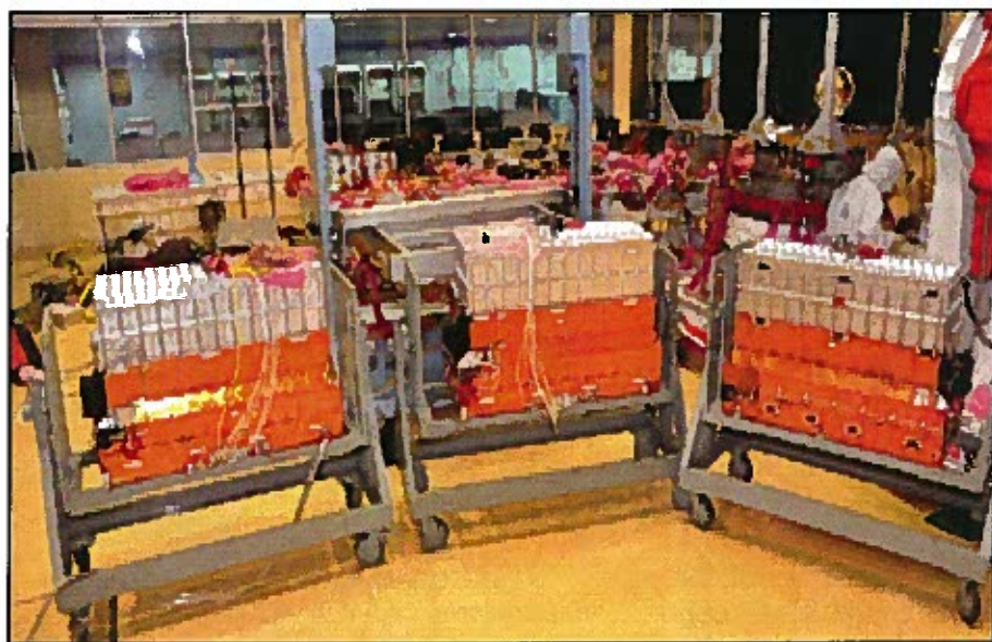
All the three LAXPC Space flight detectors in Assembly, integration and testing lab (AIT) lab after successfully completing all flight tests and final calibration (20 th October 2014).
